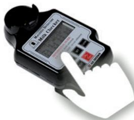
Press the «TEST» button. The display shows the absolute value of the electrical conductivity (ABS) of the teat on the upper left of the screen.
