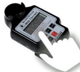
Press the «TEST» button again in order to display the difference in electrical conductivity (DIF).
